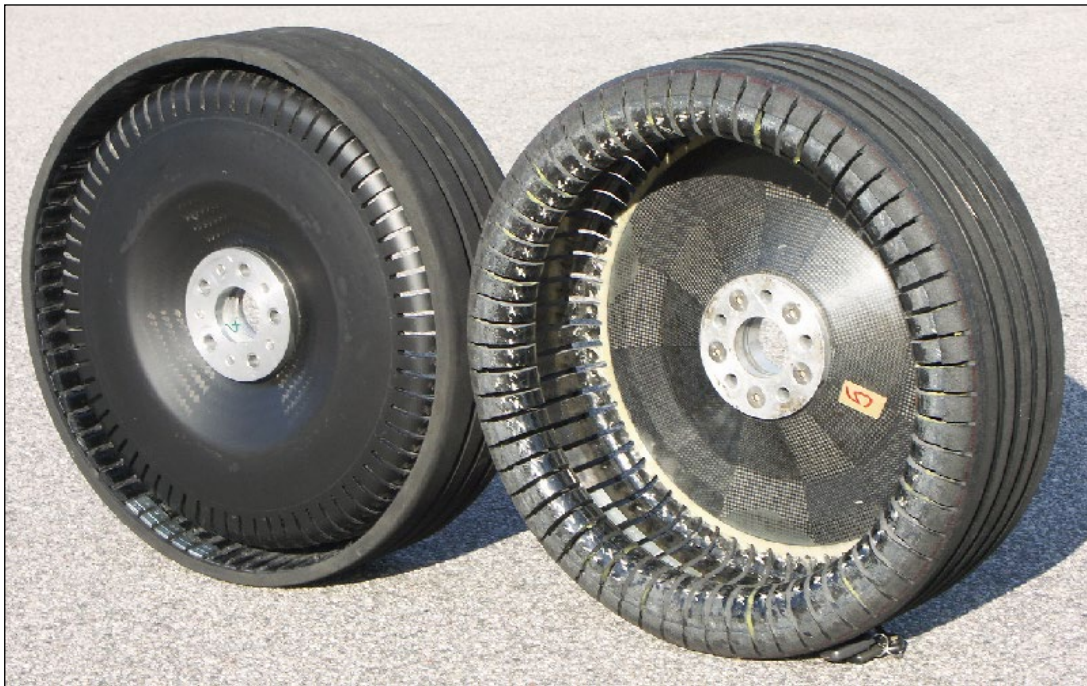
Figure 1: The Composite Wheel according to the last version produced in an earlier project. The left half shows the side facing outwards from the car, the right half facing inwards. From [7].
