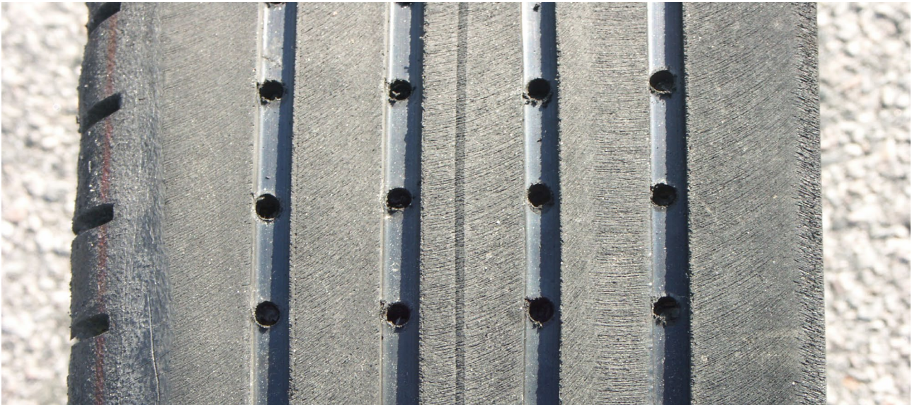
Figure 2: The tread shown from above. Note the circular holes at the bottom of the longitudinal grooves which are drilled through the belt. The holes have a diameter of 6 mm and are 30 mm apart.
